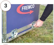
Loosen all four butterfly latches (Two on each side).
