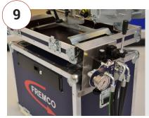
The control valve can be be hung on the edge of the box. You can then access the control valve from the operational part of the machine.
