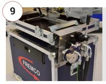
The control valve can be be hung on the edge of the box.
