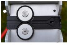
For micro cable size 3.0 - 4.5 mm MAX adaptor plates and MAX steel wheel applies.
